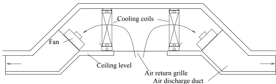
FIGURE 2. Cross sectional view of penthouse evaporator design in end elevation.
