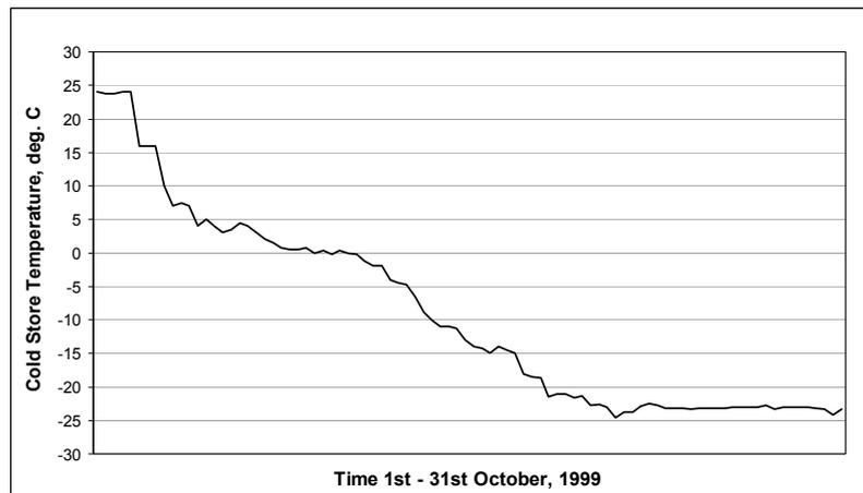
FIGURE 4. Temperature pull-down as a function of time following completion of the facility.
