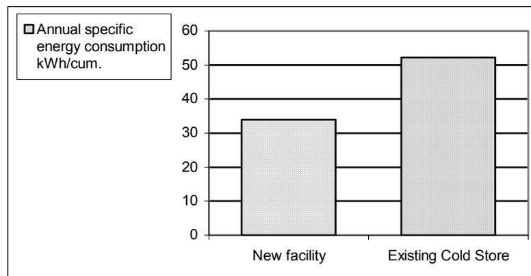
FIGURE 6. Annual specific energy consumption in  $\text{kWh}/\text{m}^3$  of storage volume including annexes for an existing cold store and the new cold store.
