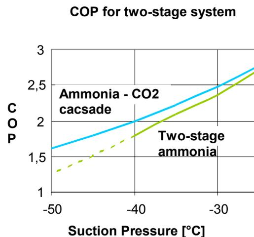
Fig. 3. COP comparison between ammonia two-stage plant and CO<sub>2</sub>/ammonia cascade plant at various compressor suction pressures (shown as saturation temperatures)
