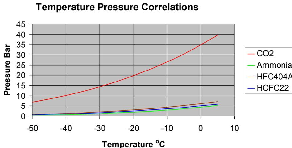
Fig. 1. Temperature – pressure relationships for different refrigerants.
