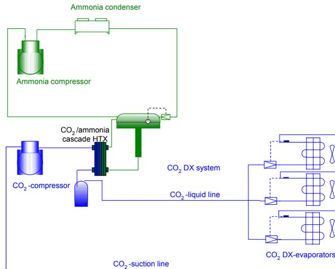
Fig. 2. CO<sub>2</sub> compressor system with dry expansion evaporators
