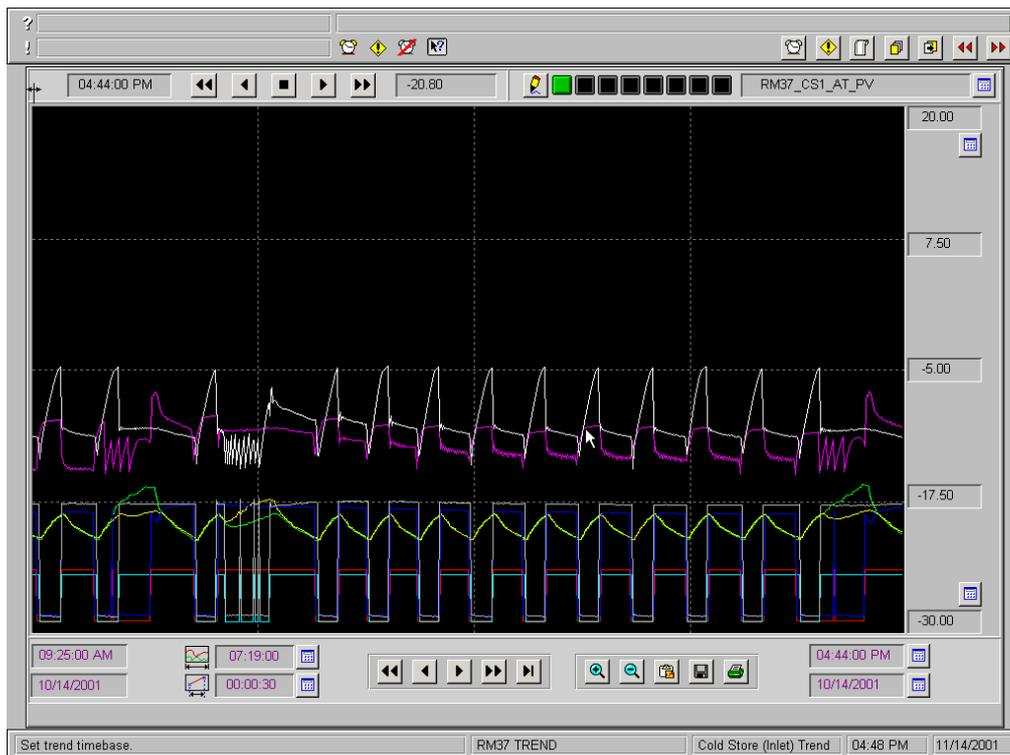
Fig. 7. Graph describing typical R744 system operating cycle
