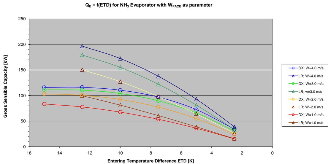
Fig. 4. Capacity for NH<sub>3</sub> evaporator as a function of entering temperature difference and face velocity. Dry expansion (DX) and liquid overfeed (LR), air on constant at -35.0°C.
