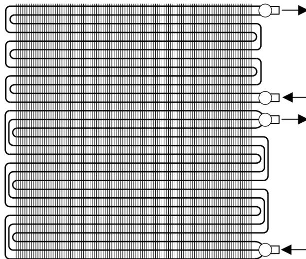
Fig. 1. Introduction of multiple headers for circuit length reduction
