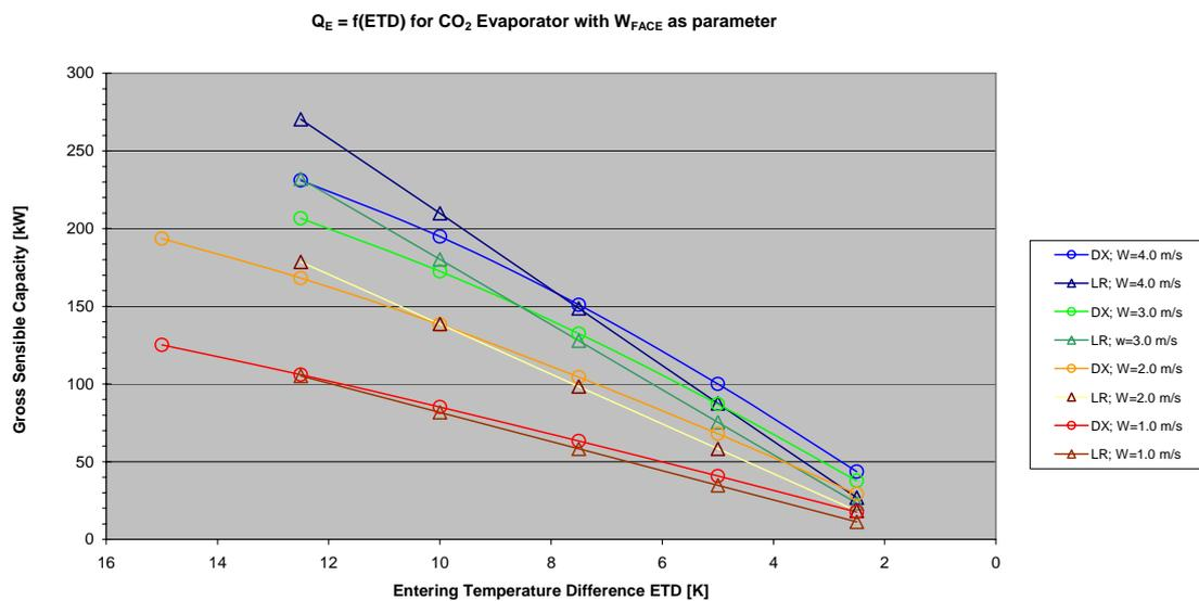
Fig. 5. Capacity for CO<sub>2</sub> evaporator as a function of entering temperature difference and face velocity. Dry expansion (DX) and liquid overfeed (LR), air on constant at -35.0°C..
