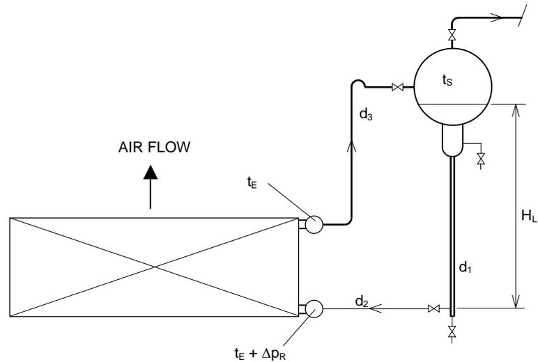
Fig. 3. Evaporator with gravity flooded refrigerant feed.
