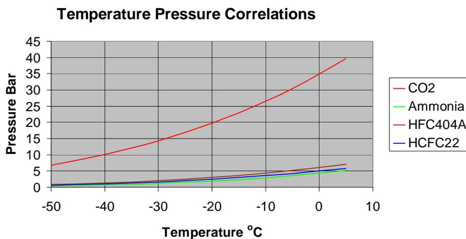
Fig. 8. Temperature – pressure relationships for various refrigerants.
