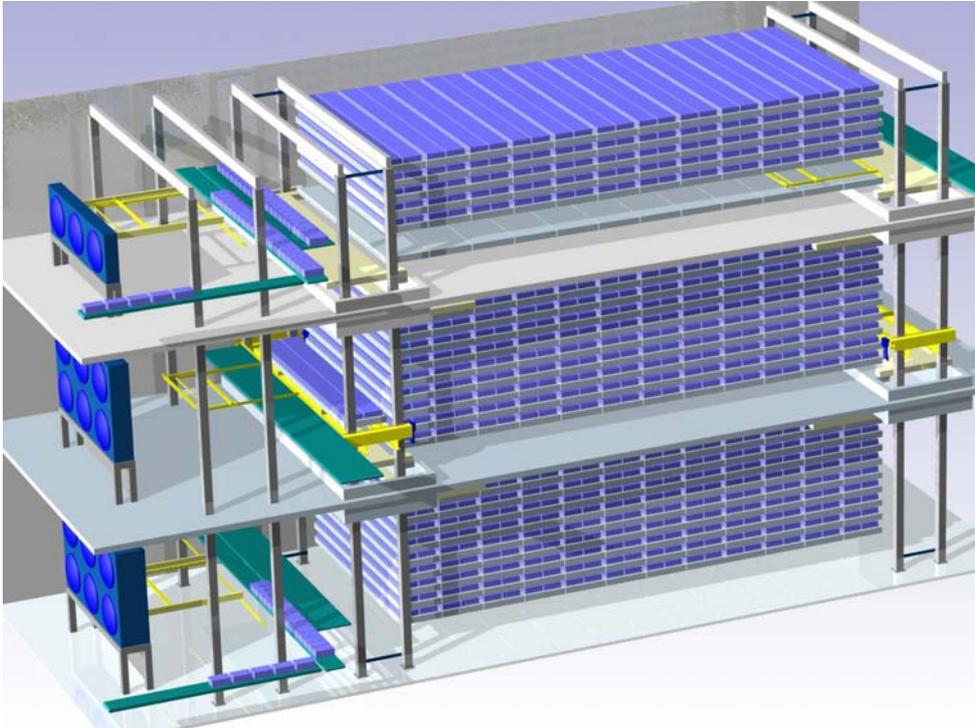
Fig. 2. Automatic TriZone air blast chilling/freezing tunnel
