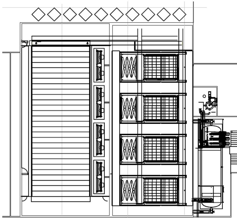
Fig.1. Conventional carton chilling/freezing plant in plan view.
