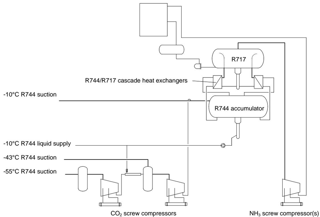
Fig. 4. Cascade type NH<sub>3</sub>/CO<sub>2</sub> refrigeration system with three temperature levels
